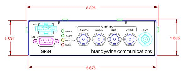
The GP4 provides access to all of the I/O, power, and signal connectors at the front of the chassis. A description of the various connectors and indicators follows:
